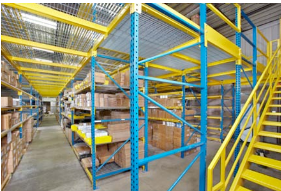
Pallet rack components are used to support a work platform above, with beam levels below for standard pallet rack storage. The upright frames can extend through the work platform floor to provide more storage levels above.
