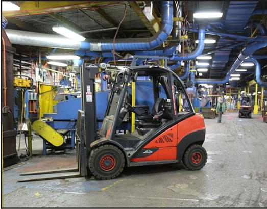
Prior to incorporating Linde forklifts into their operation, the facility encountered damage to exposed hoses, as well as issues with brakes, steering linkage, motors and tire wear. The forklifts would frequently go into failure around 8,000 hours.
